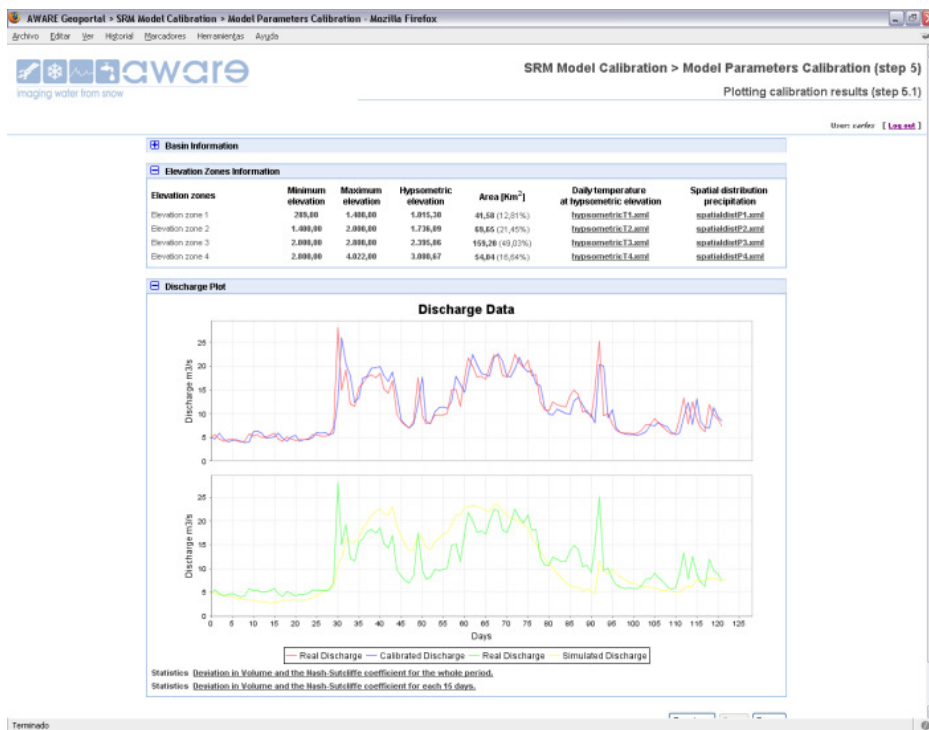
Figure 56. Results with plots comparing calibrated, real and simulated discharges of the watershed.
