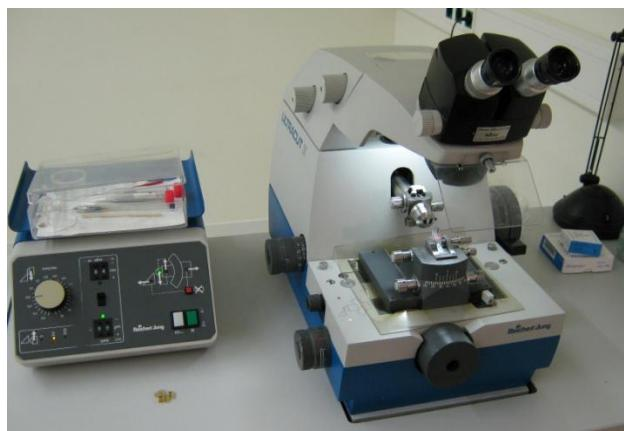
Figure 44. Ultramicrotome Reichert-Jung Ultracut E
