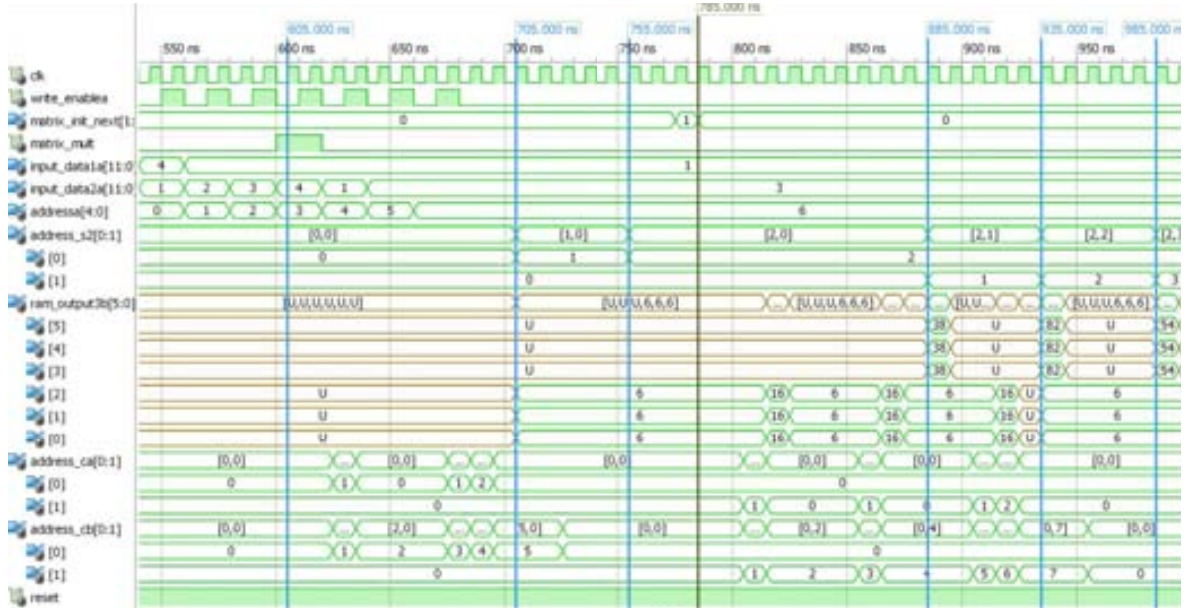
Figure 5.12: Simulation of Matrix multiplier \mathbf{A} \times \mathbf{B} \times \mathbf{C} implemented in VHDL.
