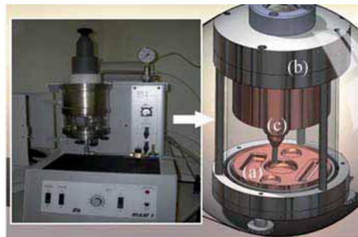
Figure 17: Left: Picture of the arc melting device used [200]. Right: Schematic representation showing (a) – copper crucible, (b) – shells with a roof on top, and (c) – retractable tungsten electrode.
