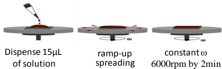
Fig. 2.3. Schematic of the spin coating solution deposition
