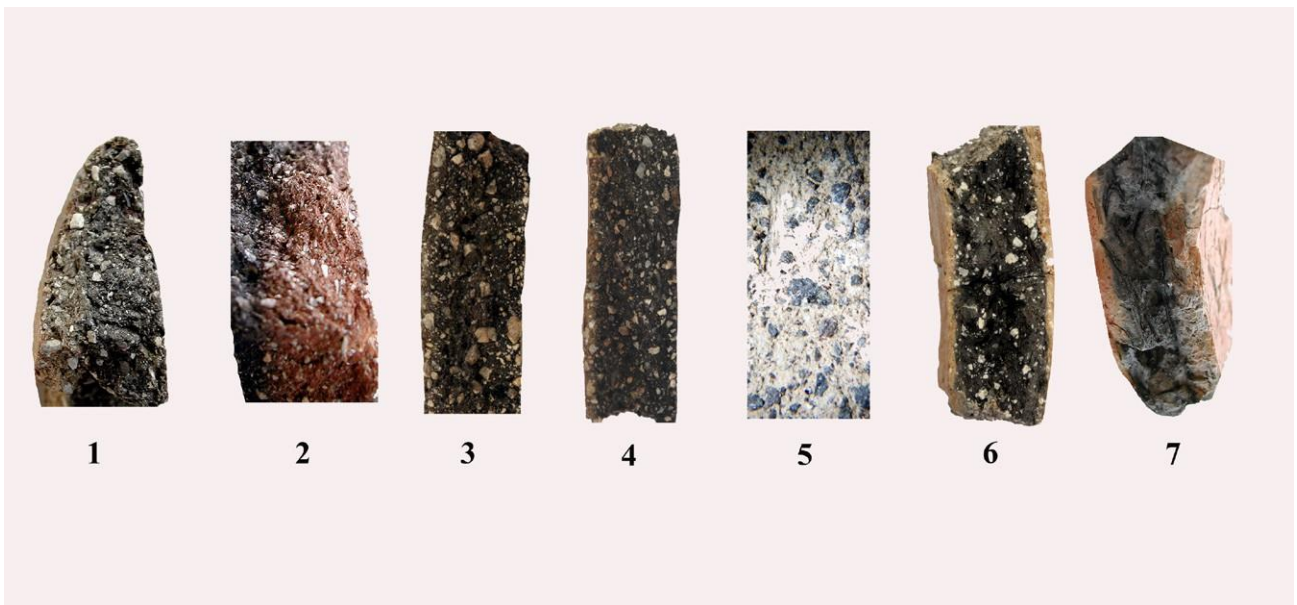
Fig. 4.9. Nature of the inclusions. 1 and 2, calcite grains; 3 and 4, calcite and sand; 5 basalt grains; 6 calcite and plant, and 7, plant and mineral.
