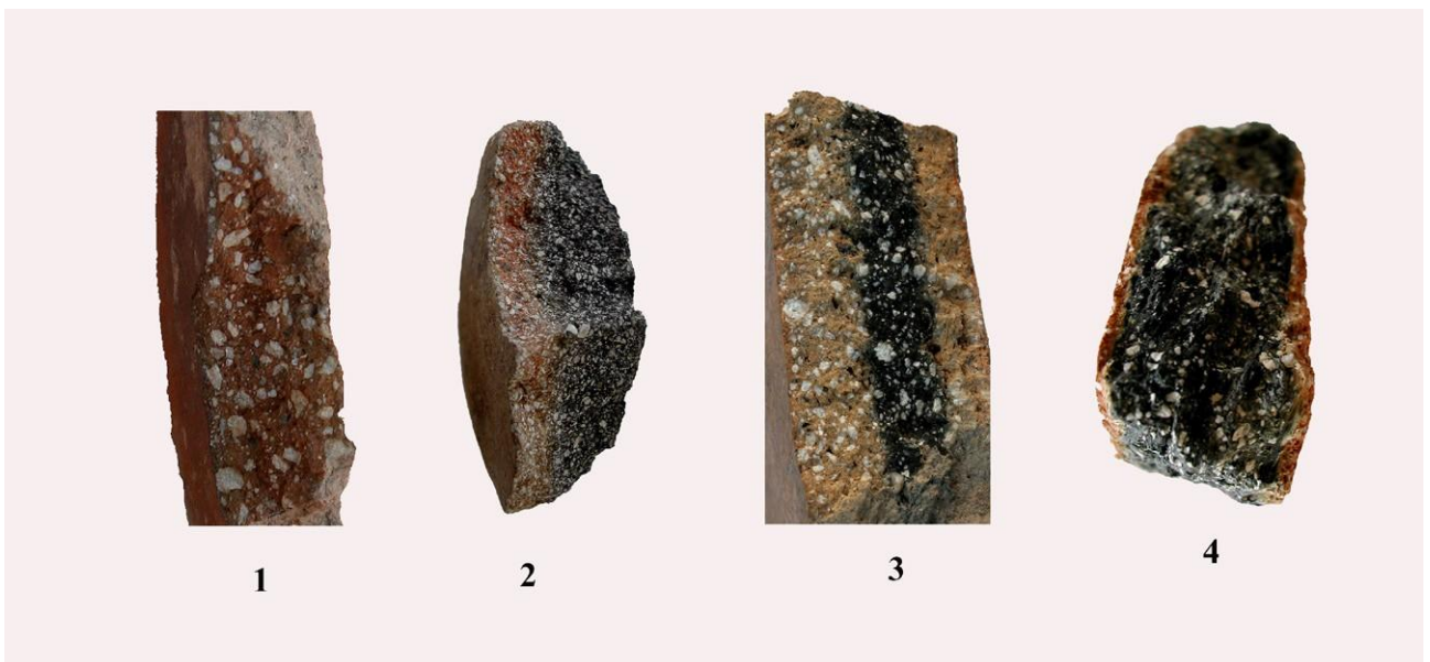
Fig. 4.10. Detail of the more representative conditions of firing; 1, oxidising; 2 and 3, oxidising/reducing and 4 reducing atmosphere.
