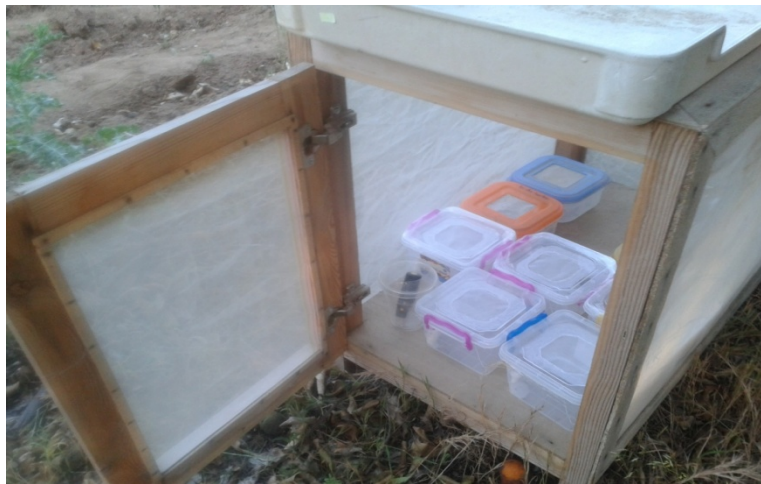
Figure 5.6. Diachasmimorpha longicaudata adult longevity determination system. The wood-framed cage was protected with a rigid plastic cover as shelter for rain. A data logger was placed inside to determine the climatic parameters of each season.
