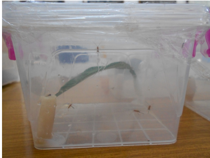
Figure 5.9. Experimental dispositive (unit) to assess D. longicaudata adult susceptibility to selected pesticides.
