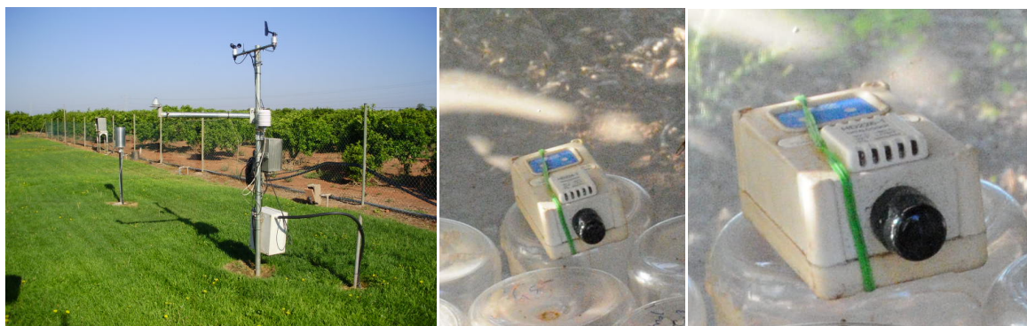
Figure 3.2. The climatic station at the IVIA research fields, and data logger used to record temperature and relative humidity inside the wood framed mesh cages used for the trials.
