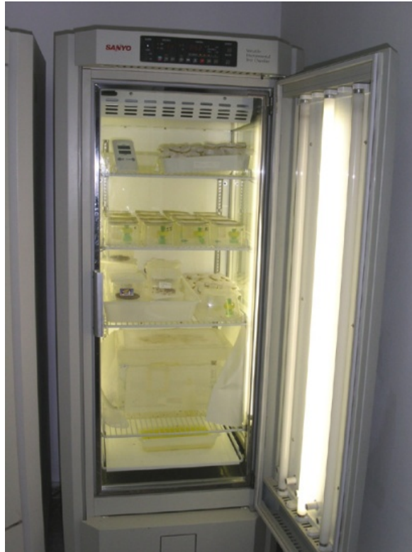
Figure 2.11. SANYO climatic chamber with temperature, humidity and photoperiod control used to determine effect of temperature on adult longevity.
