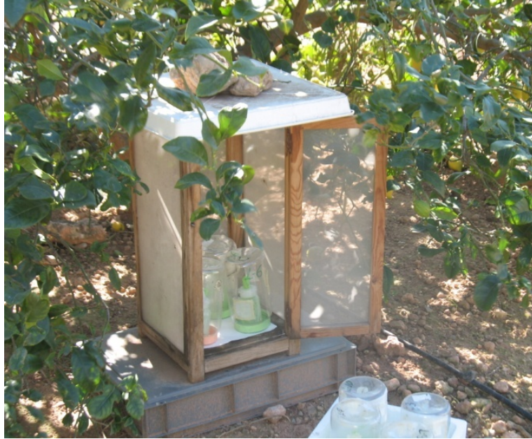
Figure 2.13. Field cage used to determine D. longicaudata longevity. Wood-framed cage was protected under the shadow of a lemon tree, plus covered with a plastic roof to protect experimental units from rain.
