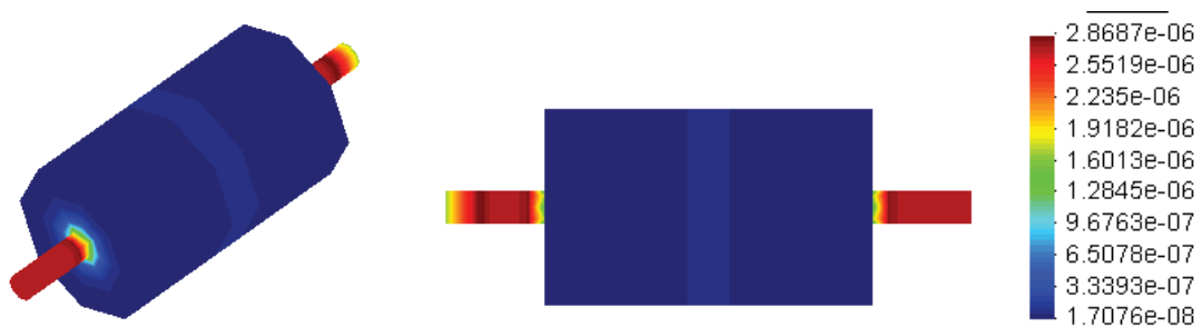
Fig. 7.26. Fluid velocity at the end of the simulation using the permeameter. On the left the coloured map of the 3D sample, in the middle a yz plane of the permeameter and on the right the scale of the colours representing the fluid velocity in m/s.
