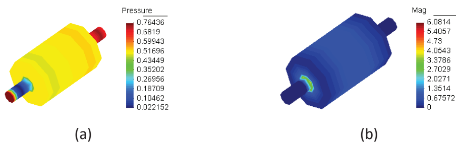
Fig. 7.27. (a) Fluid pressure at the end of the simulation and (b) drag force at the end of the simulation.
