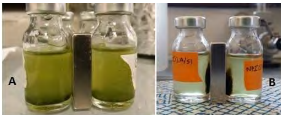
Figure 8.3. Magnetic separation of microalgae; (A) Without NPs, and (B) With \text{Fe}_3\text{O}_4 NPs-I (0.25 g/L of the NPs, and 20 min magnetic decantation time).
