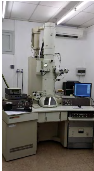
Figure 3.5. Transmission electron microscope (JEM-2011/JEOL) instruments from Servei de Microscopia at UAB.
