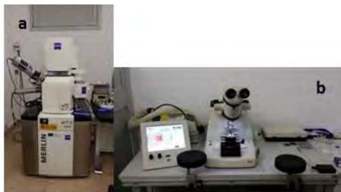
Figure 3.4. (a) Scanning electron microscopy, Zeiss Merlin, and (b) Leica UC7 ultramicrotome instruments from Servei de Microscopia at UAB.
