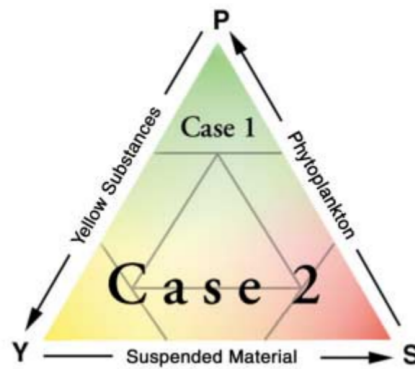
Figure 1.3: Diagrammatic representation of Case 1 and Case 2 waters. Source: Sathyendranath (2000) .
