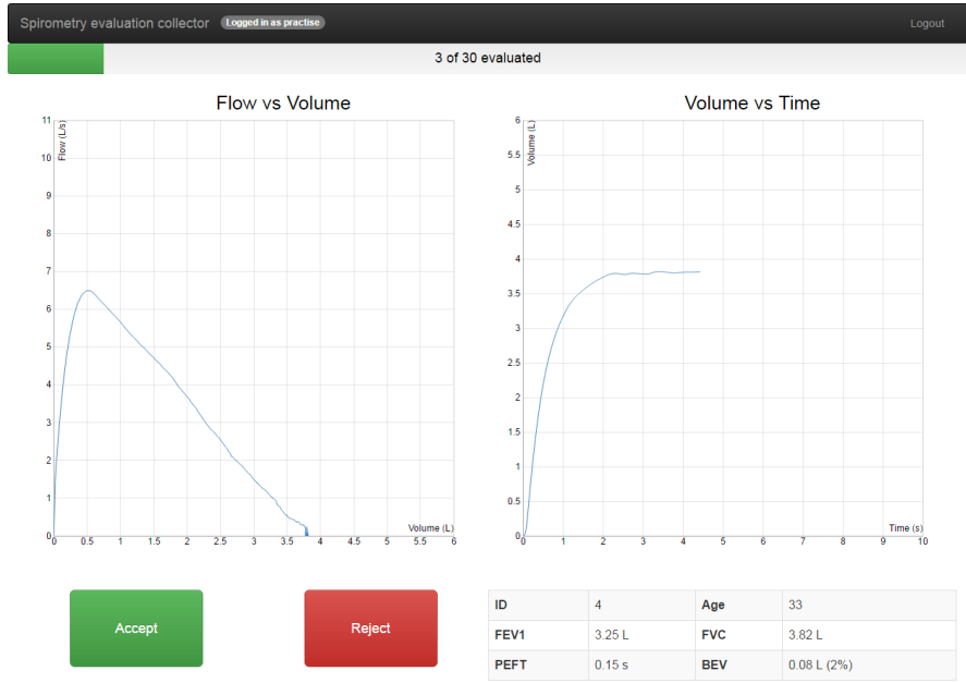
Figure 4: Spirometry evaluation collector: the spirogram quality acquisition tool.
