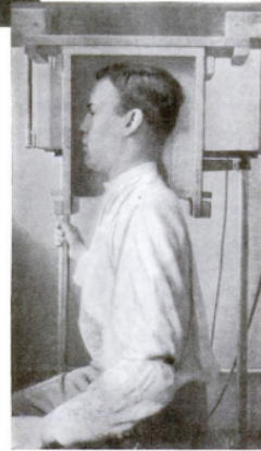
A profile mask inside the box holds the subject's head in a rigid position while X-ray photographs of his speech organs are taken.
