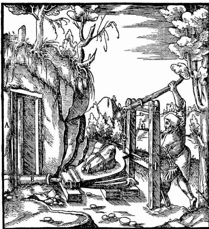
A—TUNNEL. B—PIPE. C—NOZZLE OF DOUBLE BELLOWS.
