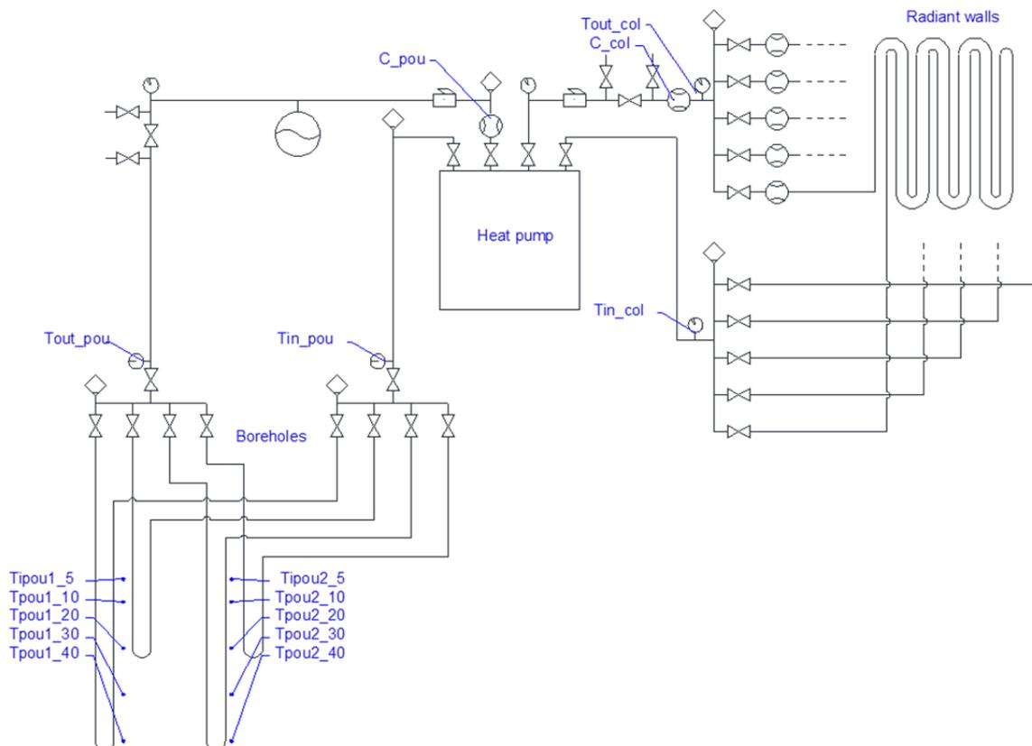
Figure 21. Distribution of sensors in the hydraulic system of the radiant cubicle
