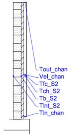
Figure 19. Distribution of sensors in the radiant wall (with ventilated facade)
