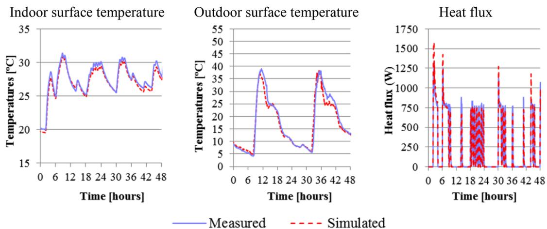
Figure 24. Comparison of the experimental data and simulation results of the East wall
