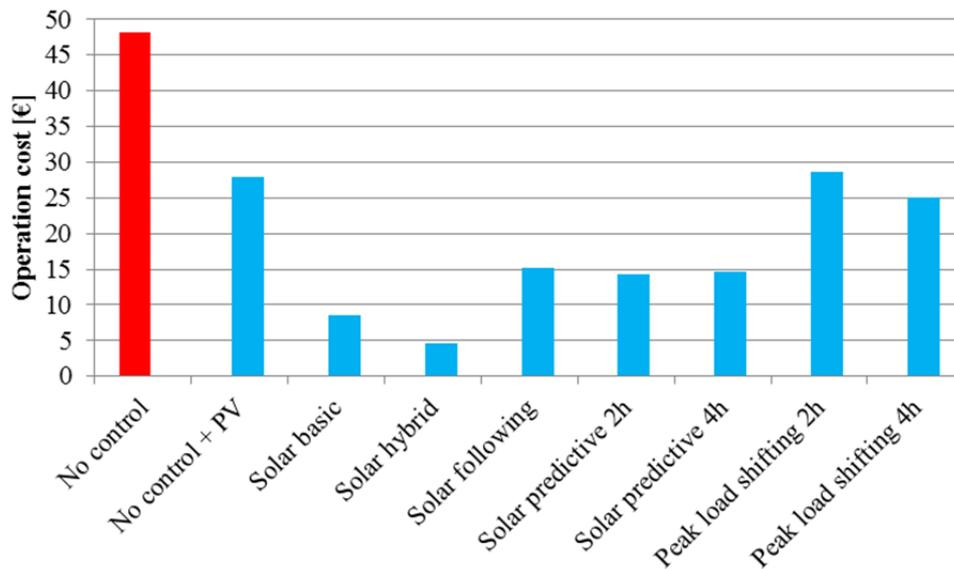
Figure 26. Operation cost of each control concepts (all “solar” concepts consider self-consumption of PV energy)
