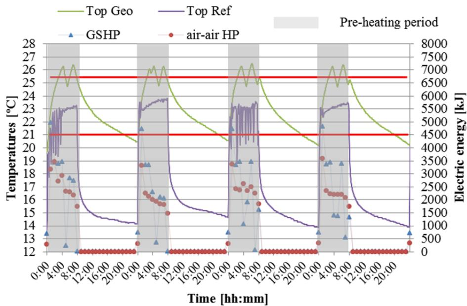
Figure 23. Temperature evolution and hourly energy use in night-time heating test
