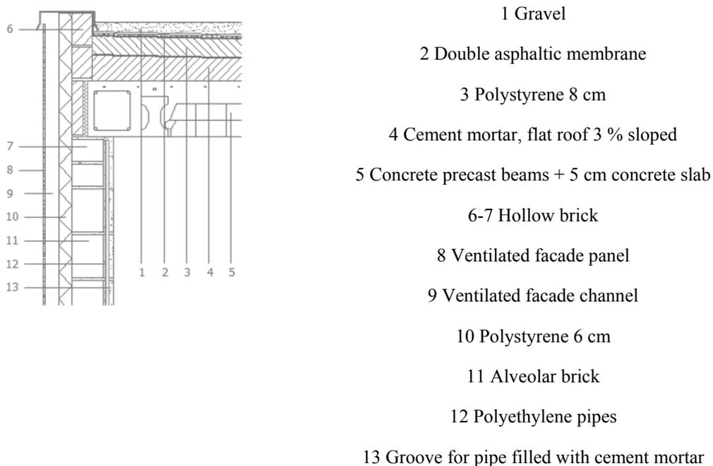
Figure 10. Roof and wall composition (with ventilated facade)
