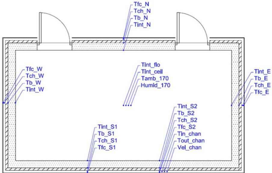
Figure 20. Distribution of temperature sensors in the radiant cubicle
