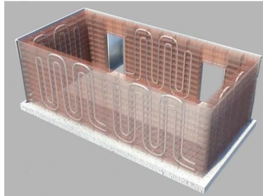
Figure 14. Scheme of radiant wall loop
