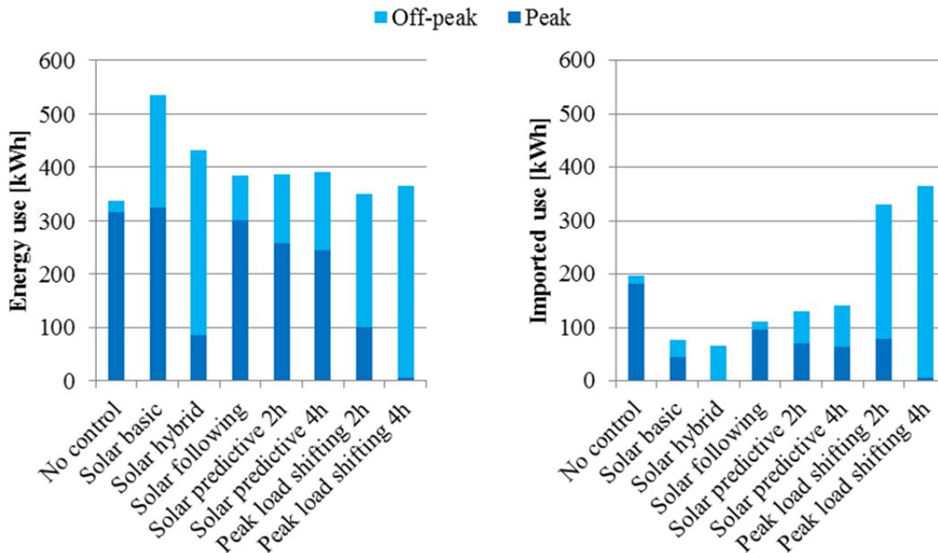
Figure 25. Total peak and total off-peak energy use (left) and imported energy (right) (all summer)
