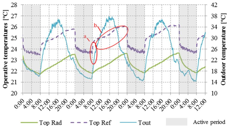
Figure 22. Operative temperatures of radiant cubicle (rad), reference cubicle (ref), and outdoor temperature during night-time operation test
