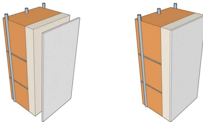
Figure 17. Schemes of the radiant wall with ventilated facade (left) and without (right)
