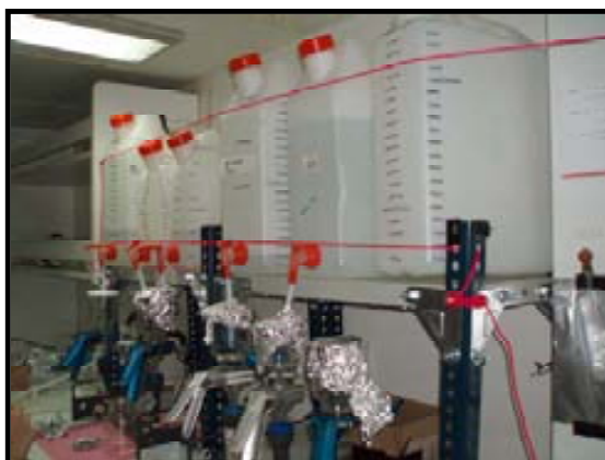
Figure 2.5. Filtration system used to sample the seawater onboard Cornide de Saavedra, March 2006.
