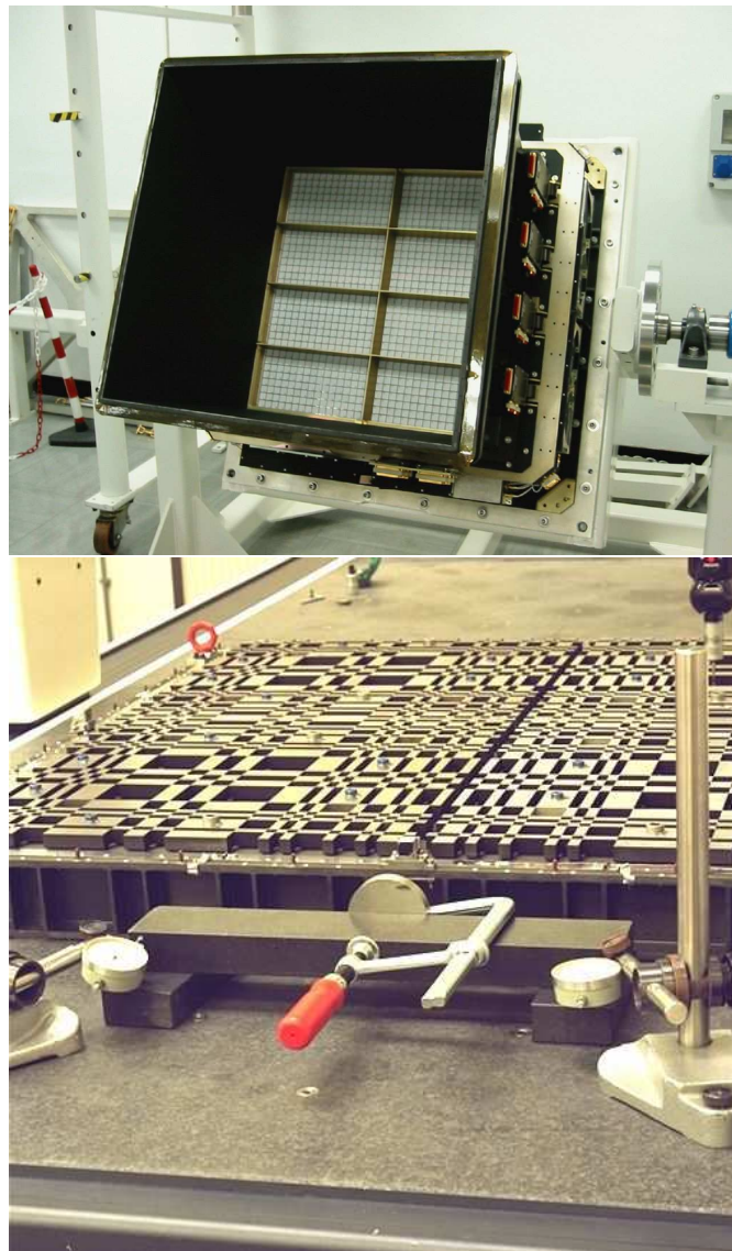
Figure 1.3: IBIS detectors (top) and coded mask (bottom). Credits: ESA.
