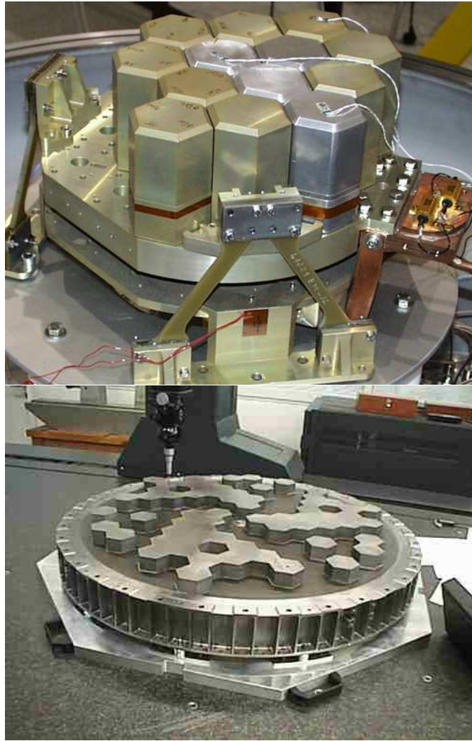
Figure 1.4: SPI detectors (top) and coded mask (bottom). Credits: ESA and CESR.
