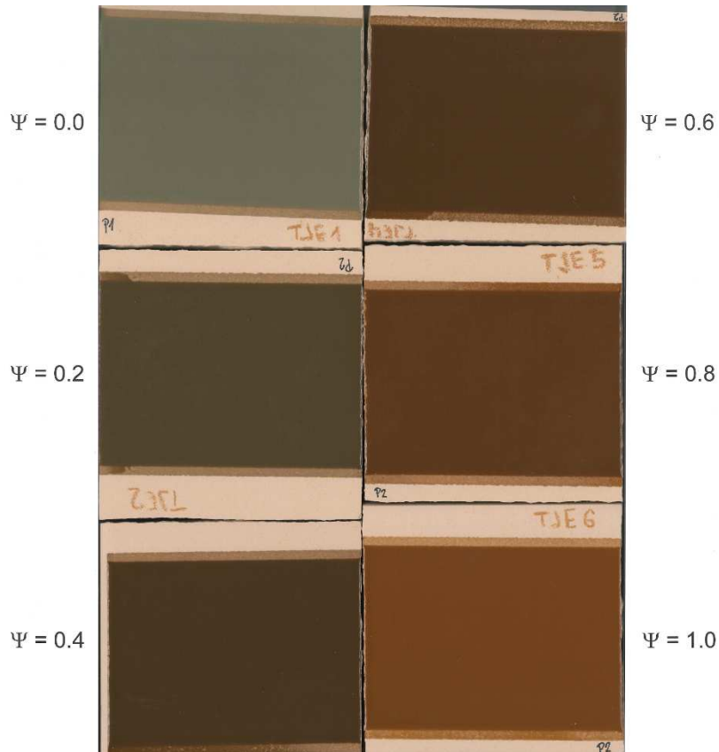
Figure 8 Example of glazed as-synthesized samples showing saturated colours with no defects on the surface
