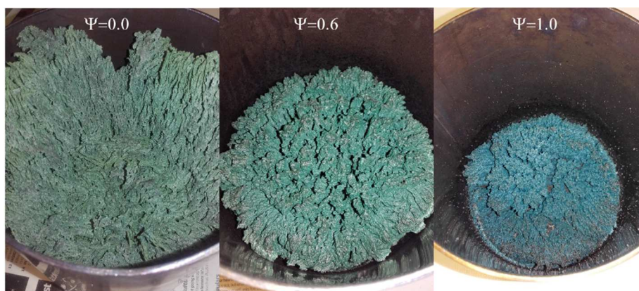
Figure 1 Images showing spinel spongy aspect evolution at three different composition steps ( T_0 = 500 °C)
