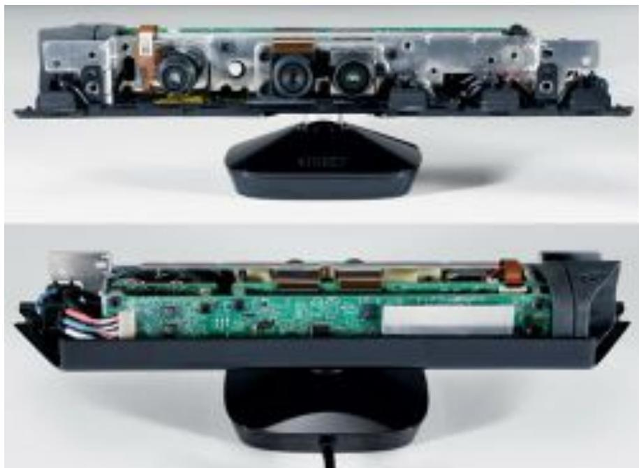
Figure 2.2: The Kinect systems is constituted of a hardware that merges a camera a depth sensor and a matrix microphone and a specific software development kit that allows to detect speech, facial expression, gestures and position.
