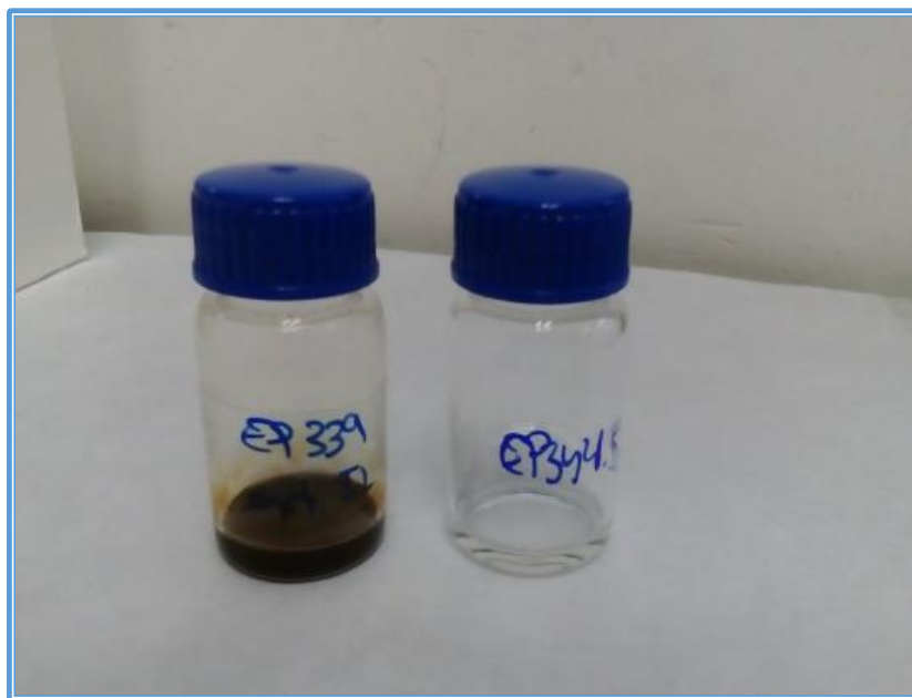
Figure S1. Et_2O (left) vs scCO_2 (right) extraction of the 3-octanone ( 6 )
