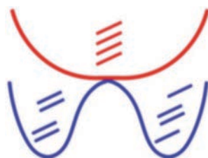
Figure 8.3: Double-Well Model showing the temperature dependence of the free energy profile (blue = low temperature, red = high temperature) associated to one column comprising four TTTA molecules with respect to an intrastack dimerization process.
