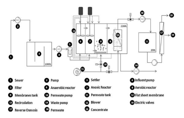
**Figure 3.1 -** Pilot plant of Castell-Platja d'Aro, treating urban wastewater with an MBR followed by a RO. Scheme taken from Dolar et al. (2012) [342].
