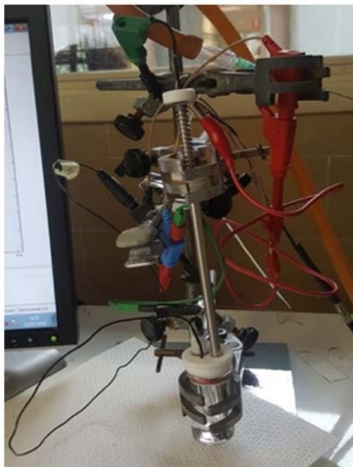
Figure 7.16: Picture of the electrochemical setup used, with a connector to be able to immerse the substrate used as the WE.
