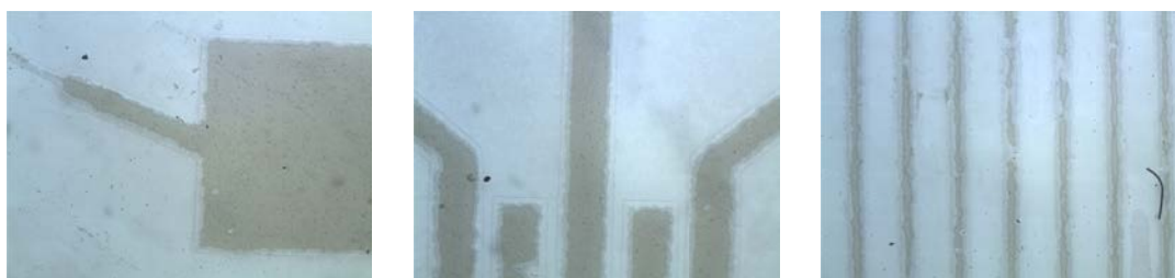
FIGURE 3.4: Optical images after ITO etching and after photomask removal. The patterned ITO electrodes are observed in dark colour with irregular borders as a result of strong underetching.
