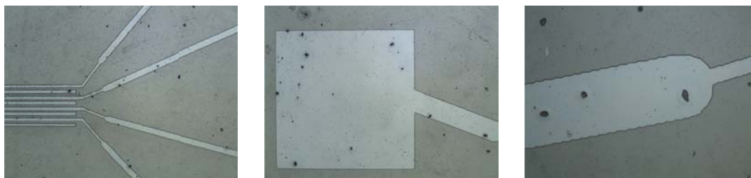
FIGURE 3.3: Optical images before ITO etching. The dark regions correspond to the excess ITO to be etched, and the light regions correspond to the photoresist-coated ITO electrodes to be patterned.
