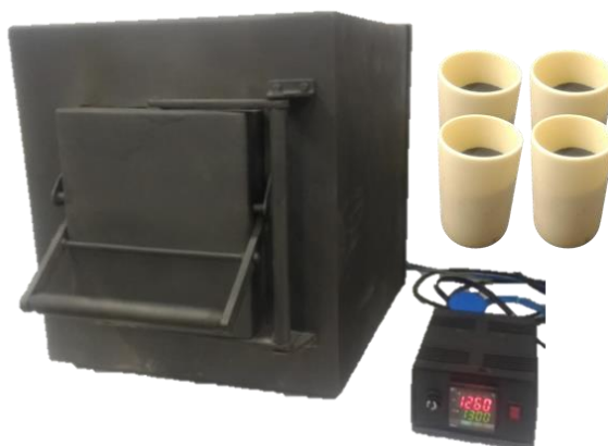
Figure 6.1. Furnace and crucibles used for thermal aging.
