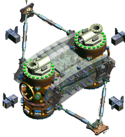
Figure 2.12: Artistic image of the LTP. The circular coils (copper color) are located next to the GRSs and the magnetometers are the grey floating boxes. Image obtained from [34].
