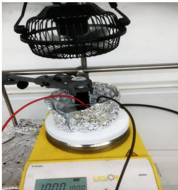
Figure III-16. Irradiation setup used in the 3 mmol-scale decarboxylative hydroalkylation of alkynes
