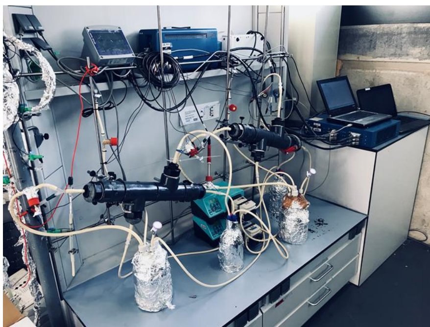
Figure 15. Real overview of the tubular duplicate reactors setup.
