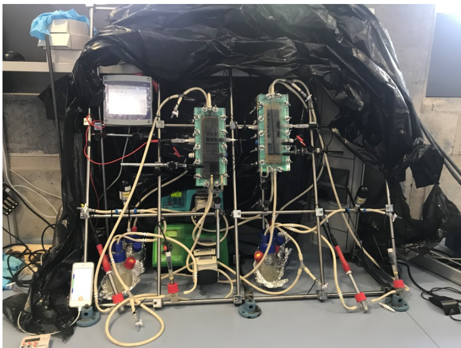
Figure 17. Real overview of the flat-plate duplicate reactors setup.
