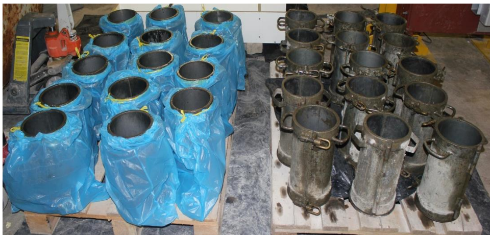
Figure 3.6 Molds of concrete specimens for short term characterization.
