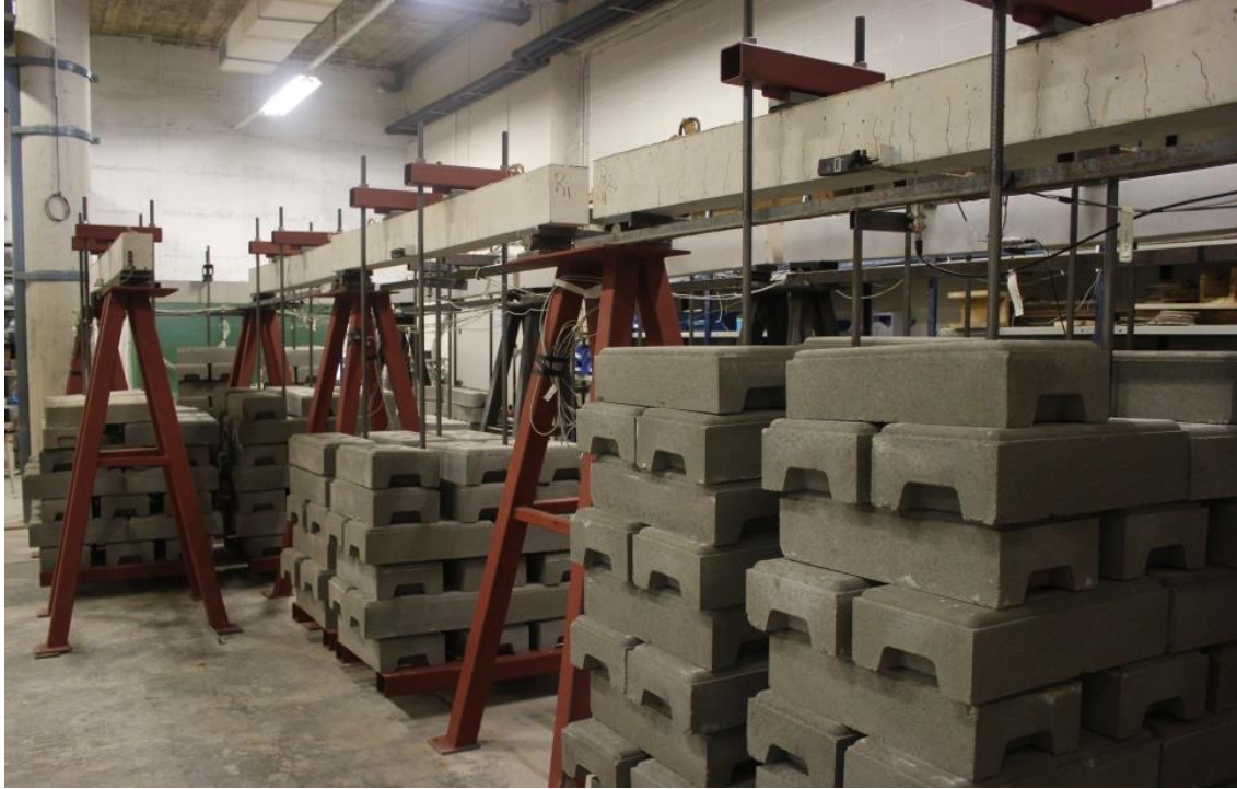
Figure 3.14 Setup and instrumentation of sustained loading test.
