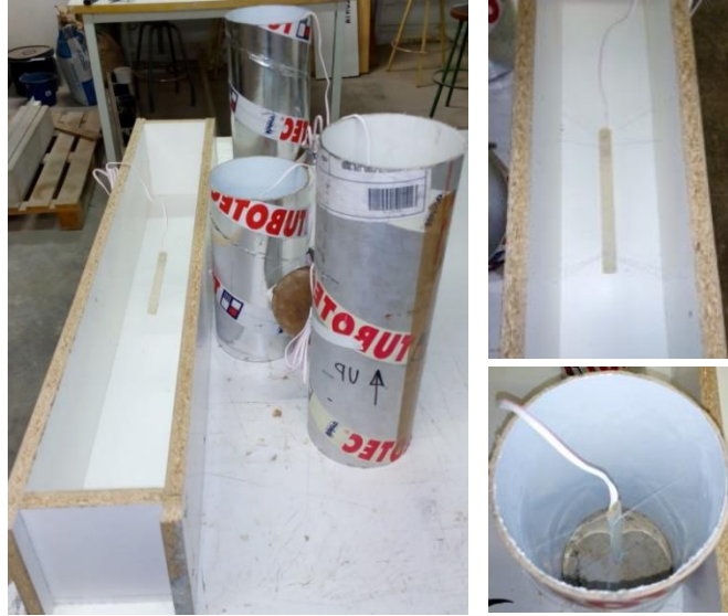
Figure 3.7 Molds of concrete specimens for creep and shrinkage and their instrumentation.
