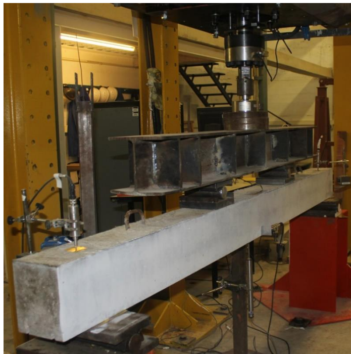
Figure 3.13 Setup and instrumentations of short-term test.
