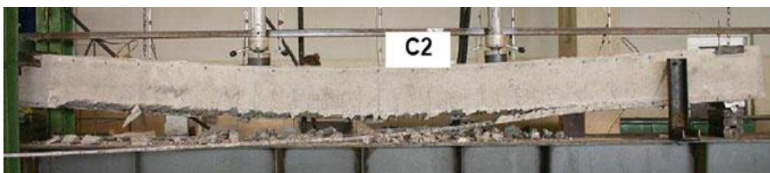
Figure 2.12 Failure by intermediate crack debonding with adjacent cover concrete [86].
