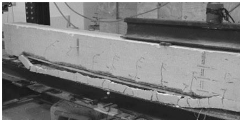
Figure 2.14 Failure by the beam edge concrete cover separation [15].
