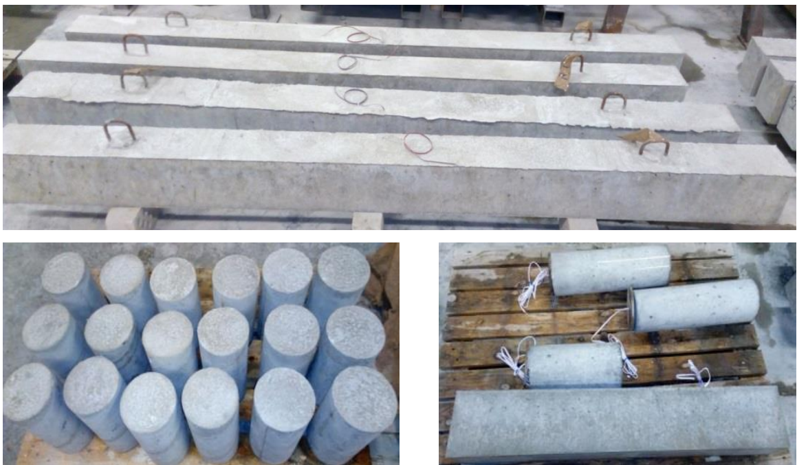
Figure 3.9 Specimens after demolding.
