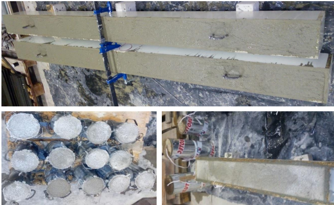
Figure 3.8 Specimens after casting and levelling.
