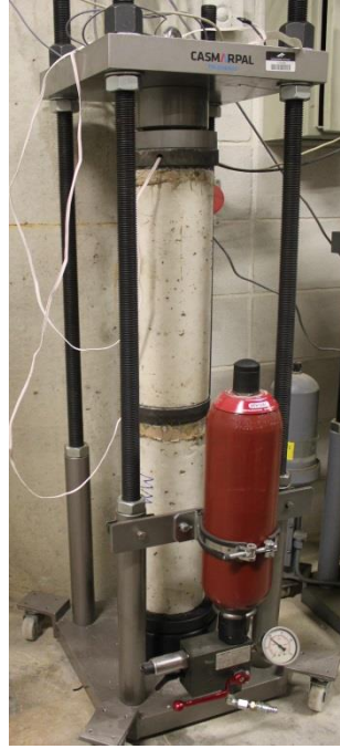
Figure 3.15 Creep load application on the concrete creep cylinders.
