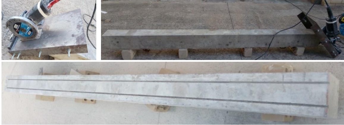
Figure 3.10 Formation of grooves.
