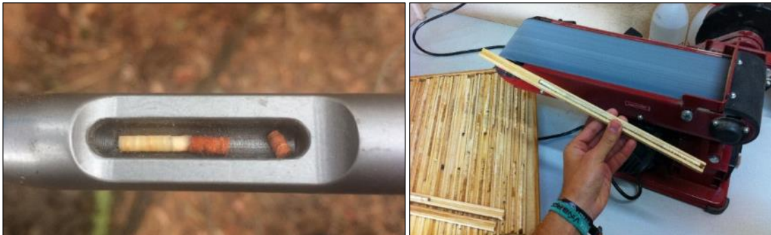
Figure 13: Extraction of one radial wood core by a Pressler increment borer (left) and polishing of the core (right).
