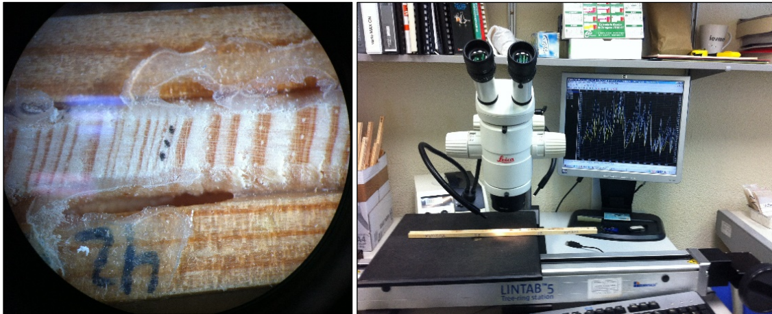
Figure 14: Visual cross-dating of wood samples and identification of latewood IADFs (left) and measuring of raw EW and LW widths by using Lintab-TSAP sliding-stage measuring device (right).
