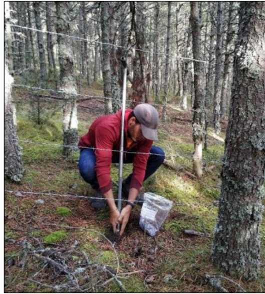
Figure 12: Extraction of soil cores by a soil sampler.
