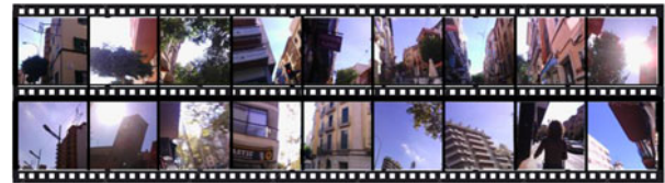
Fig. 1. Example of a sequence acquired by the narrative clip wearable camera while the user is walking down a street. The temporal leaps between neighboring pictures produced by photographic cameras are common in dynamic environments and make the extraction of information from closely spaced images very difficult.
