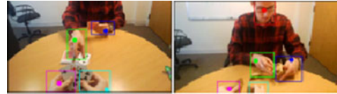
Fig. 11. Examples of first-person point of view images for recognizing activities involving hands. The algorithm is capable of detecting the left and right hands of the user, in pink and light blue, respectively, and the left and right hand of the person he/she is interacting with, in dark blue and green, respectively. Image adapted from [58], devoted to hand disambiguation.
