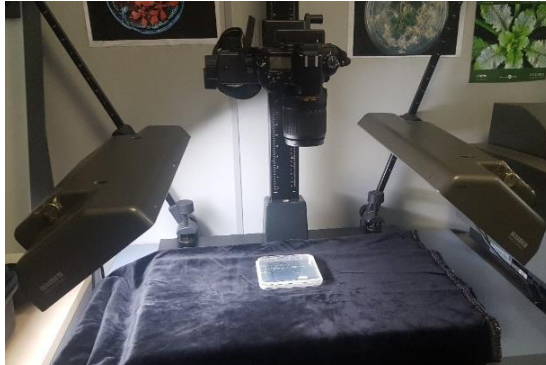
Figure 2.2: Laboratory setup for taking the pictures of the plates.
