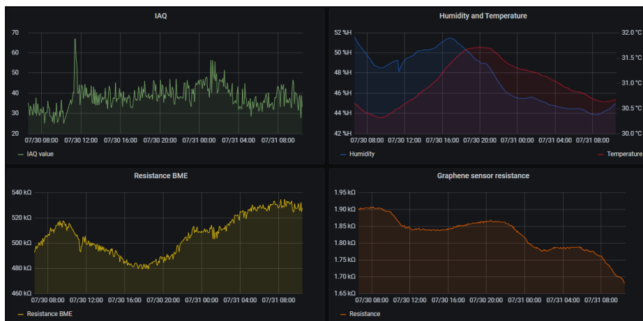
Figure S4. Graphic interface of the web service for monitoring sensor data. IAQ value calculated from the BME680 sensor (top-left), temperature (top-right), humidity (top-right), BME680 sensor resistance (bottom-left), and graphene lab-synthesized sensor resistance (bottom-right). The figure shows the same time period than Figure 11 in the manuscript.
