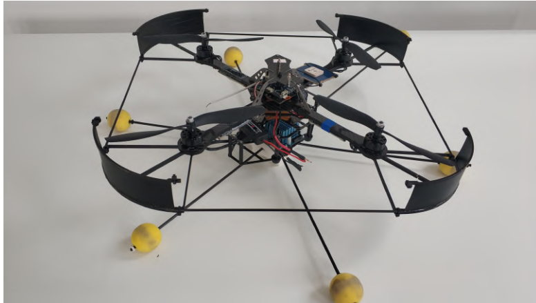
FIGURE 3.1: Asctec Hummingbird Quadrotor with the Odroid XU4Q on-board PC (center bottom of the UAV).
