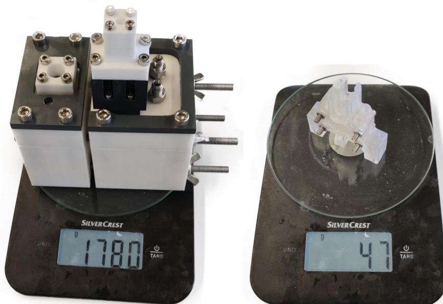
Figure 48: Weight in grams of the workshop manufactured reactor (on the left) against 3D printed reactor (on the right).
