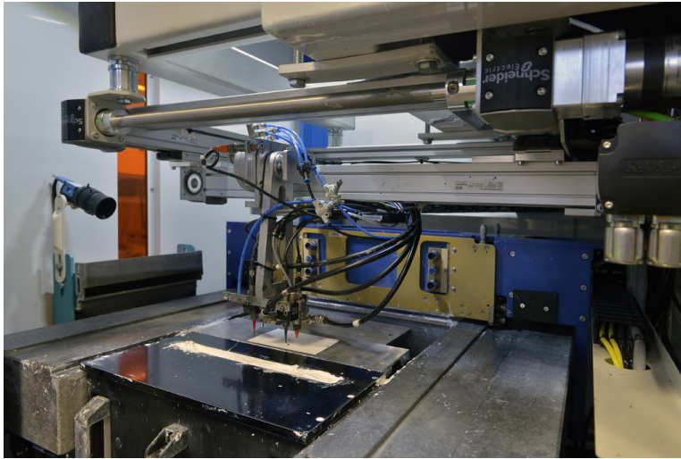
Figure 2.19: Robocasting arm in position over the printing platform.
