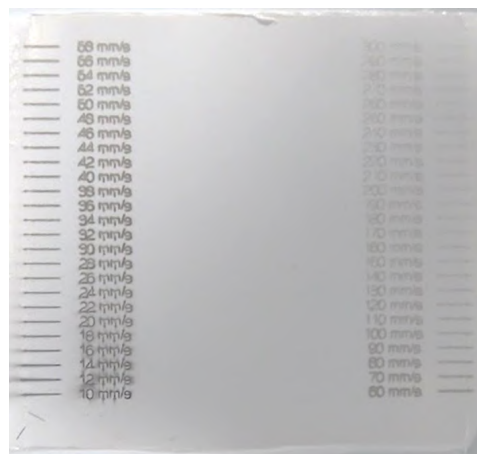
Figure 3.21: Image of an 8YSZ SLA printed part engraved with lines at different laser rastering speeds (the laser speed is specified besides each line).
