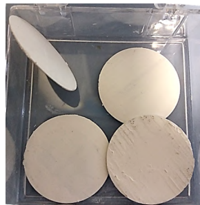
Figure B.5: Printed electrolytes based on developed 6\text{Yb}_4\text{ScSZ} paste
