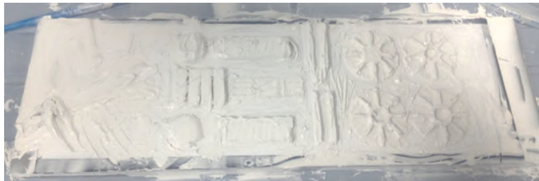
Figure 2.31: Picture of the printing platform after removing the uncured paste
