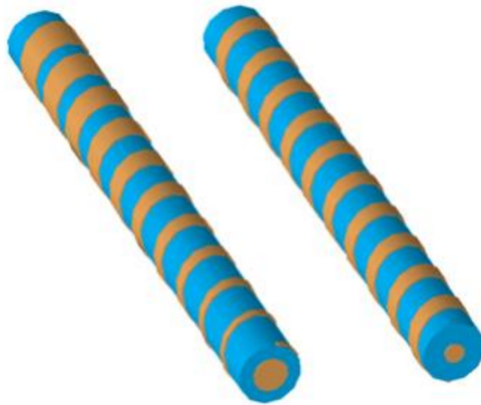
FIGURE 4.17: CAD model of the helical-microstrip impedance transformer prototypes. Left: variable width transformer. Right: conical interior conductor transformer.
