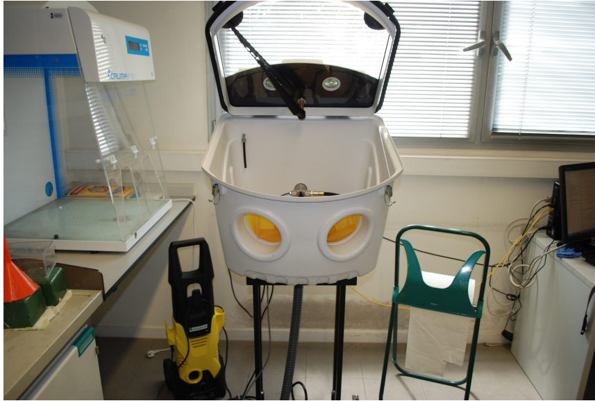
FIGURE 2.5: Pressurized water equipment for sample cleaning.
