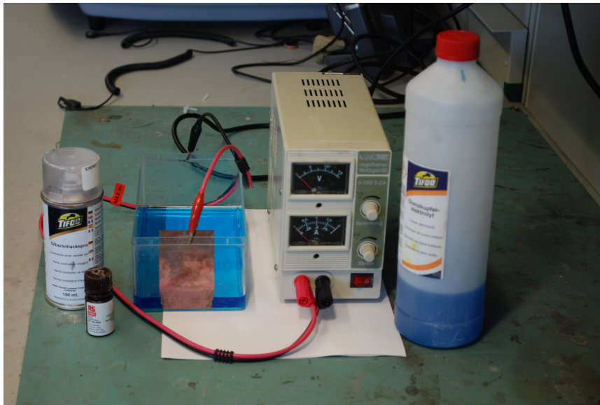
FIGURE 2.7: Equipment for the electroplating bath.
