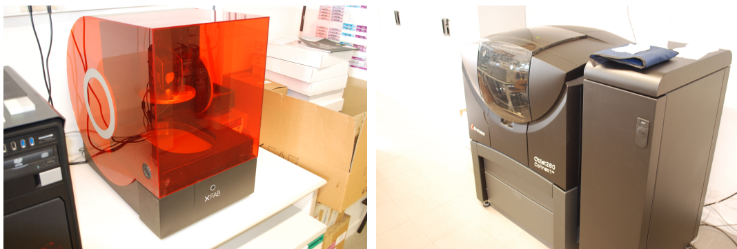
(A) XFAB 3D printer from DWS Systems.
