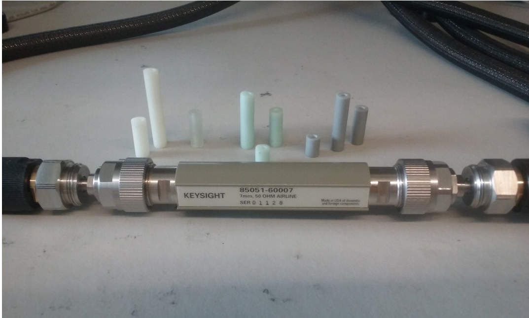
FIGURE 2.16: 85051-60007 Coaxial waveguide, 7 mm, 50 ohm, from Keysight Technologies Inc. The upstanding cylinders are the samples, made with the DWS Systems printable materials Invicta 915, Therma 289 and Precisa 779, from left to right.
