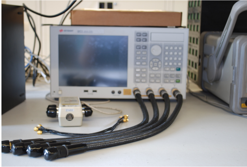
FIGURE 2.14: E5071C 4-port VNA from Keysight Technologies Inc.
