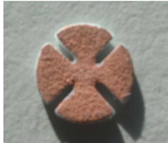
(B) One of the metallized Van der Pauw samples used in the experiments.
