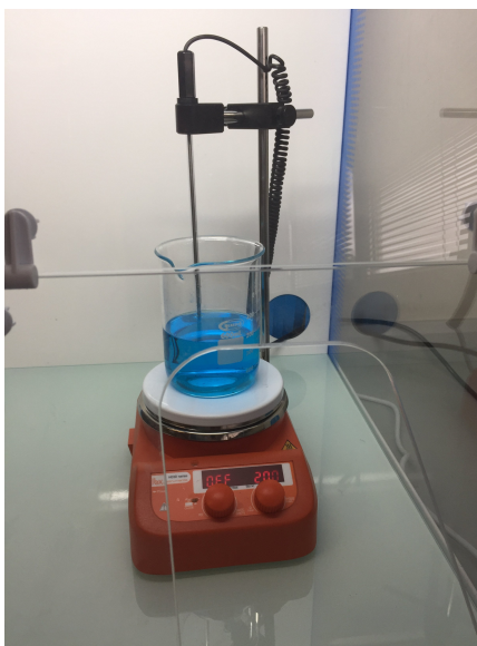
FIGURE 2.6: Equipment for the electroless bath.
