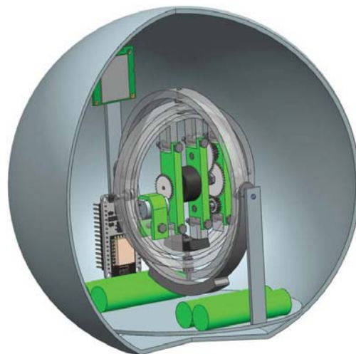
Fig. 5. Sketch of the kinetic EH placed inside an undrogued drifter, with battery pack, antenna and electronics.
