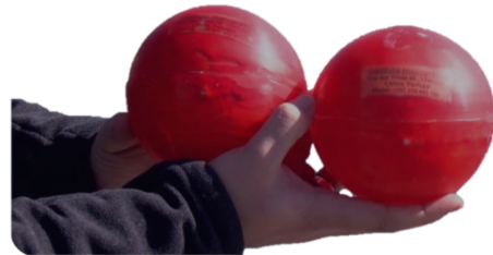
Figure 1. MELOA coastal WAVY drifter design for sea monitoring.
