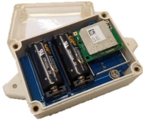
Fig. 5. TD1205P module encapsulated with two CR123A 3V batteries within an IP64 case (83×35×57 mm).
