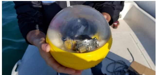
Figure 7. Oceanic drifter with the KEH, the measuring electronics and the communication system on it.
