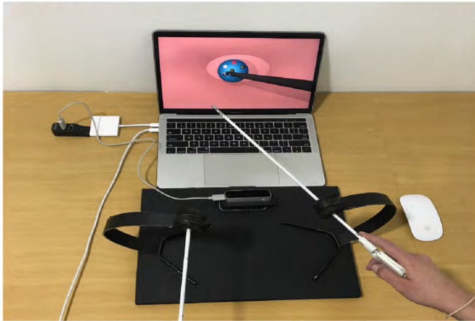
Figure 4. The final version of the simulator once the nonelectronic hardware devices had been added: the pad and support devices for the forceps and the Leap Motion Controller.
