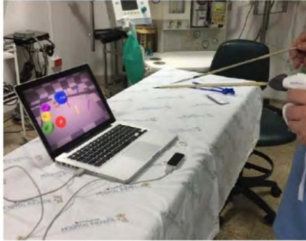
Figure 4. The final version of the simulator once the nonelectronic hardware devices had been added: the pad and support devices for the forceps and the Leap Motion Controller.
