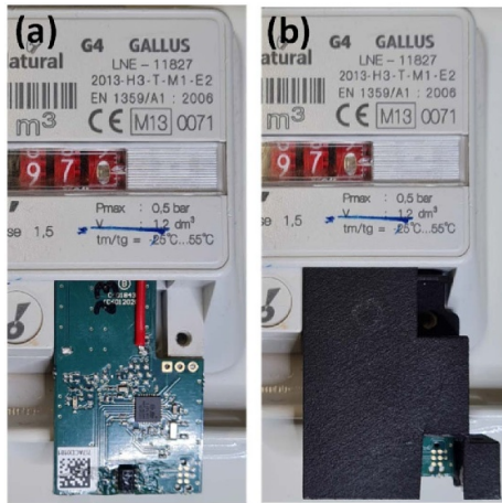
Figure 5. Placement of the PCB shown in figure 4 into the gas meter: (a) without the protecting box, (b) with the protecting box.
