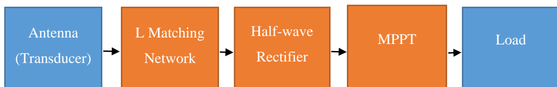
Figure 17: Particular case of the implementation of an RF energy harvester.
