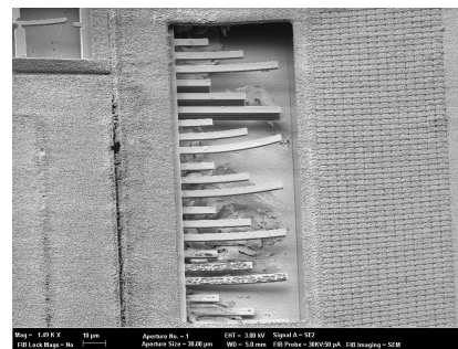
(a) Damage to the standard passivation
