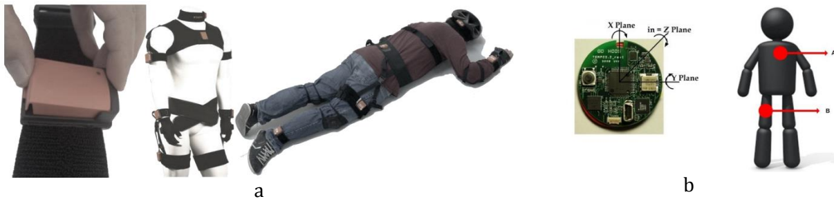
Figure 2-5 Wearable automatic safety system (a), Tri-axial accelerometer TEMPO 3.0 sensor node (Li Q. J., 2009) and placement
