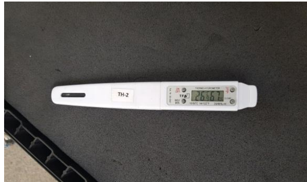
Figure 4-41 Thermometer used to measure ambient temperature and humidity-By Author
