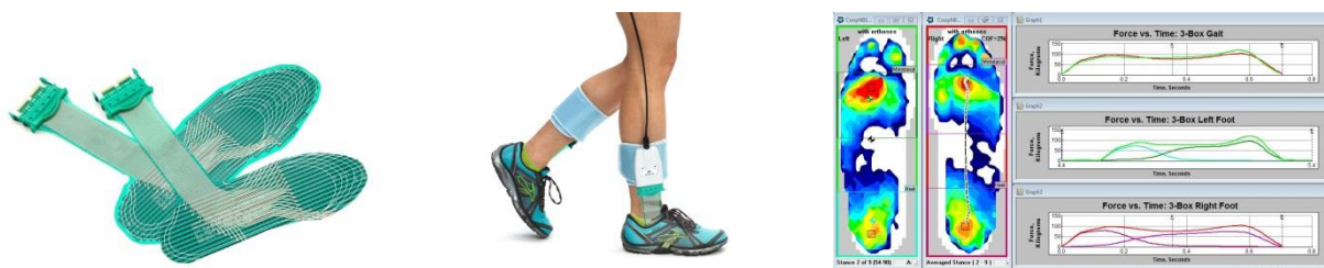
Figure 4-47 insole pressure sensor system (Tekscan, Tekscan, 2019)
