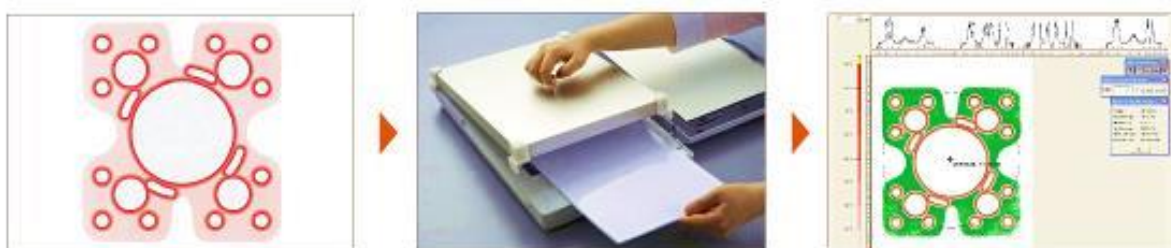
Figure 3-23 Prepare the colored prescale → Scan Prescale samples → Perform analysis utilizing FPD-8010E software 67
