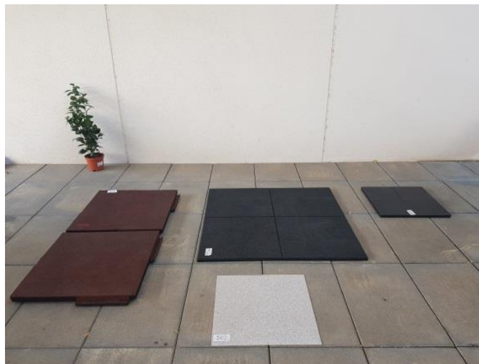
Figure 4-40 Pavements used in the HIC test-By Author
