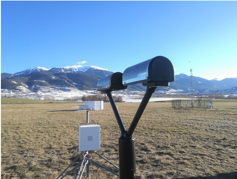
Fig. 1.3: OTT Parsivel 2 disdrometer from University of Barcelona (center) and an automated weather station from the SMC (right) located in Das, La Cerdanya (Pyrenees).
