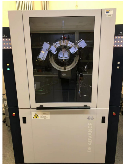
Fig. 2.3.1. The Bruker-AXS D8 X-ray diffractometer used in the present work.
