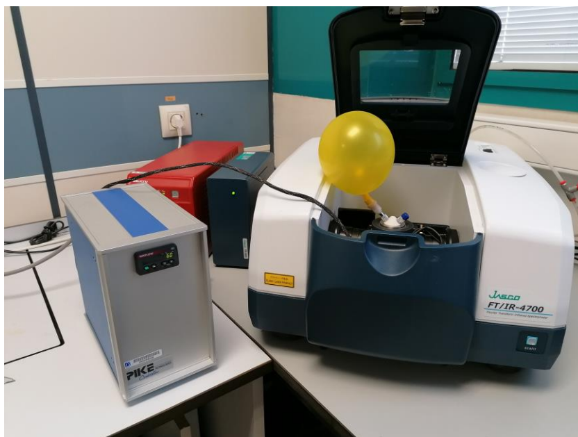
Figure S7.5. Experimental set-up for the FTIR spectroscopy kinetic analyses. The temperature was maintained constant at 60 °C with the aid of an auxiliary peltier. CO 2 was introduced in the system with a balloon. The reaction was performed under solvent-less conditions.
