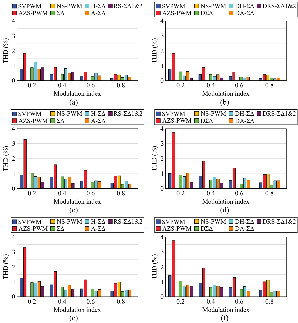
Figure B.7 Experimental THDs of PWM and \Sigma\Delta modulations on the GaN converter at different switching frequencies. (a) and (b) THDs at 100 kHz. (c) and (d) THDs at 200 kHz. (e) and (f) THDs at 300 kHz.
