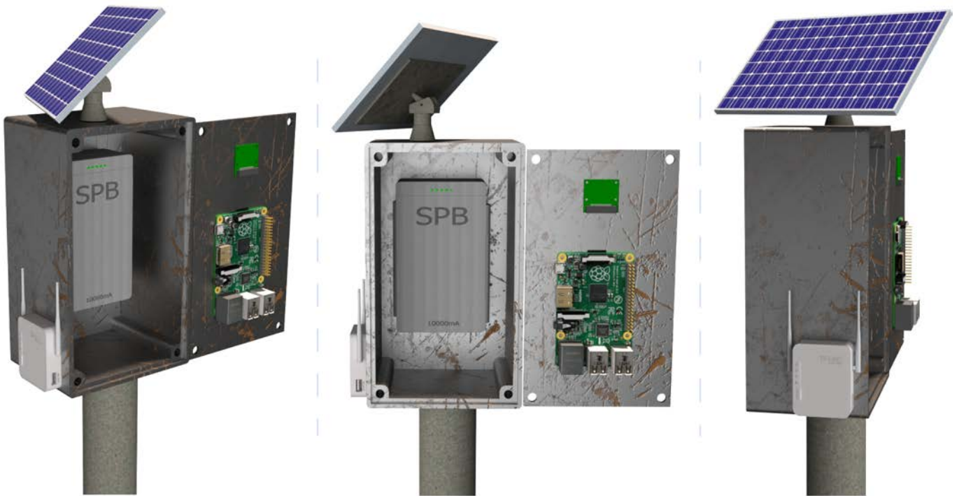
Figure II.10. Rendering of the RasPi system. Includes the basic elements such as the solar panel, the powerbank, the control unit and the Raspberry Pi Camera.
