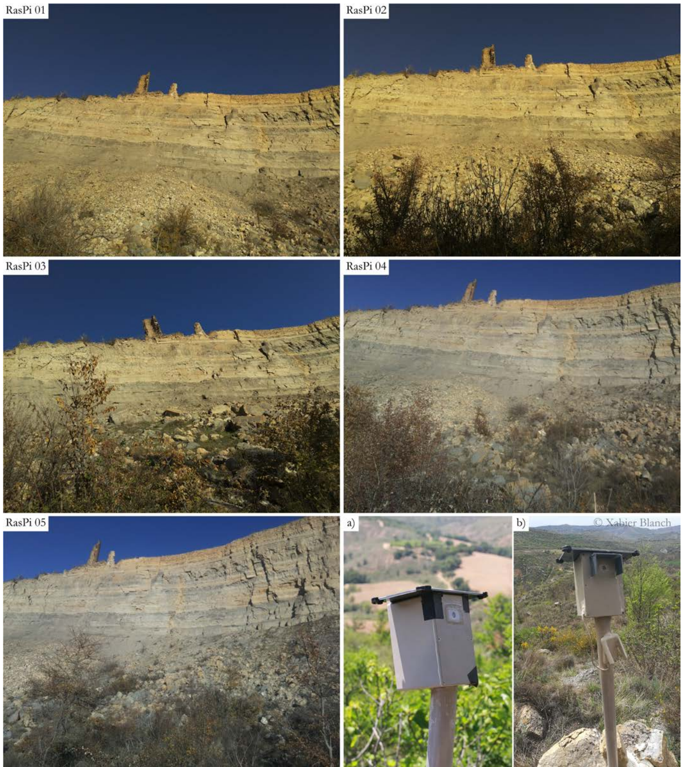
Figure III.2. Images obtained with each photogrammetric system on 29 November 2019 at 15:45h. a,b) Recent images of the RasPi system. The difference between image a) and b) is the installation of the external Wi-Fi antenna to improve signal reception.
