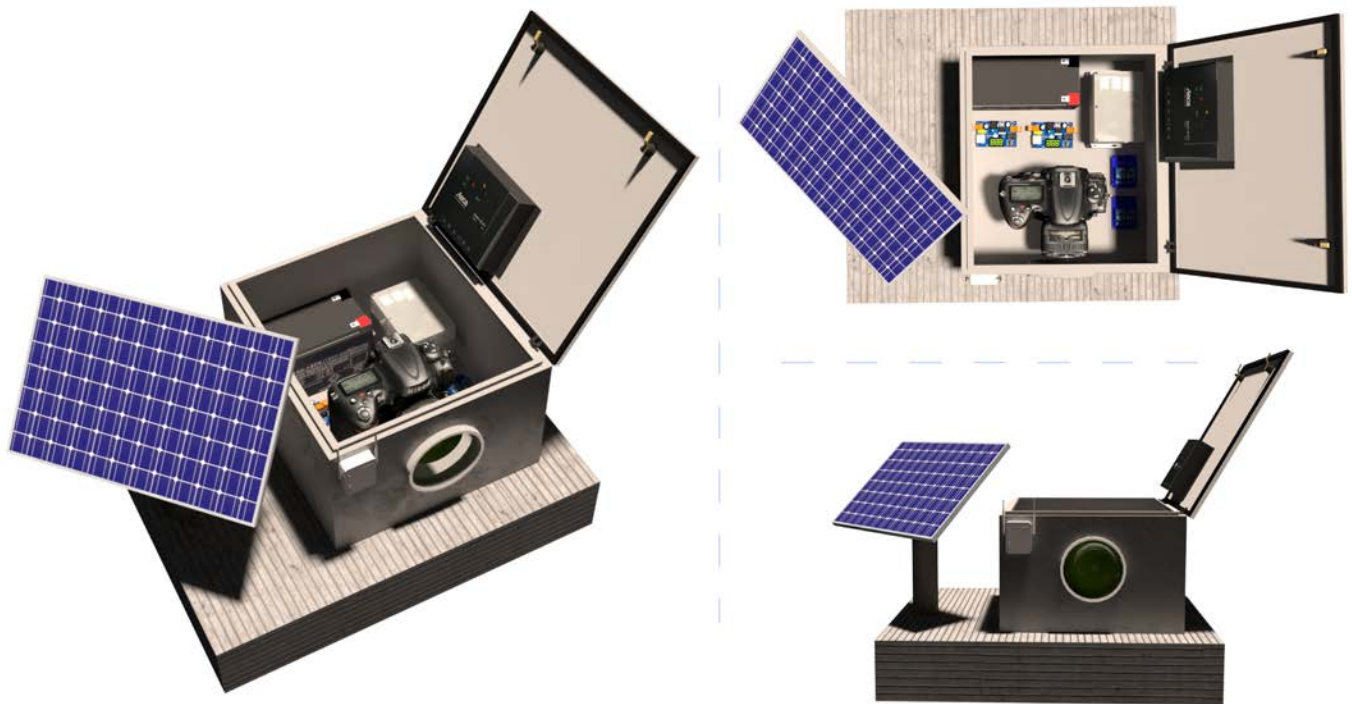
Figure II.16. Rendering of the HRCam system. Includes the basic elements such as the camera, lense, solar panel, solar charge regulator, AGM battery, relays, DC-DC converters and the control unit.
