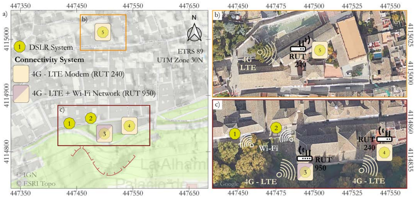
Figure II.24. Location of the 3 connectivity systems installed in Granada-Alhambra. Numbers represent the photogrammetric system. IGN and ESRI Topo base map and Google Maps images. a) Global location map. b) System located in the Escuela-Hogar. c) Systems installed in the Church of San Pedro, Zafra Convent and Archaeological Museum. QR17 (next page) show images of the devices installed in Granada.
