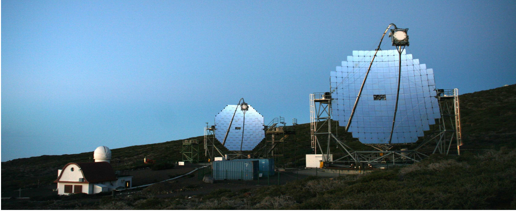
Figure 7.4: MAGIC telescopes at El Roque de Los Muchachos in the canary island of La Palma, Spain. The MAGIC I telescope is on the left, the MAGIC II telescope on the right. The small building at the left corner of the picture is the counting house where the operation of both telescopes is realized.
