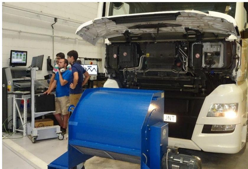
Figure 5.4. Vehicle being tested on the rolling bench.
