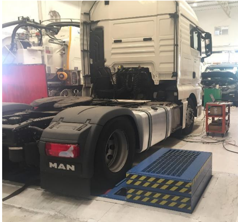
Figure 4.7. Vehicle position on the rolling bench during the experiment.
