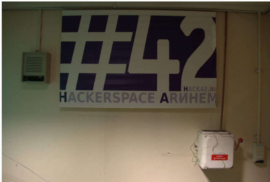
Figure 24: Door system switch, on the bottom right, Hack42 hackerspace in Arnhem, The Netherlands. Original legend reads (emphasis mine): “Hack42 Spacestate switch. Flip the switch to the ‘on’ position and the entire building will come to life . The ‘open’ spacestate will be twittered, displayed on our website and the IRC channel.” Licence: CC-BY-SA 2.0 Unported. Author: Dennis van Zuijlekom. Source: https://www.flickr.com/photos/dvanzuijlekom/6556630813/in/pool-hack42
