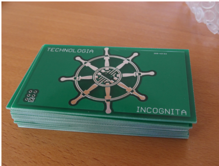
Figure 26: Etched TechInc logo PCB, ordered from factory. Licence: All Rights Reserved. Used with the permission of the author. Author: Brainsmoke. Source: https://wiki.techinc.nl/index.php/File:Test_batch.jpg
