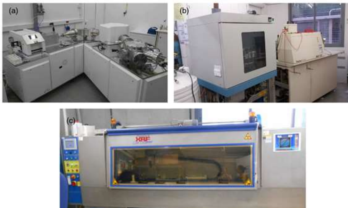
Figure 2.7 – Images of the used instruments in this study: a) Plasma 3 Multi Collector Inductively Coupled Plasma Mass Spectrometer (Nu Instruments-AMETEK) at Centres Científics i Tecnològics of the Universitat de Barcelona (CCiT-UB). Picture courtesy of Panthalassa. b) Finnigan-MAT 252 mass spectrometer at CCiT-UB. c) Avatech III Core Scanner system at Facultat de Ciències de la Terra. Pictures b and c courtesy of J. Torner.
