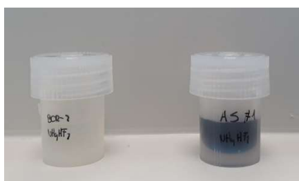
Figure 3.9 – Visual comparison of BCR-2 and ALB-2 in digestion IV Comparison done at the end of the digestion protocol IV between the BCR-2 sample (left) and ALB-2 (right). The ALB-2 sample clearly shows a remaining black residue
